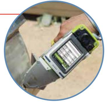
Analyze nearly every element of interest in virtually all types of metal alloys, from tramp elements to pure metals, and everything in between. With point-and-shoot simplicity, you can view the alloy grade and chemistry on the built-in, color, touch-screen display.
